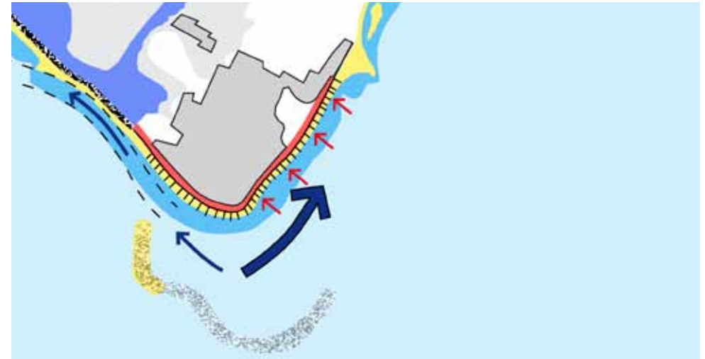
The situation in Selsey - as defined by Going Dutch II 2009 The map shows the transit of shingle from west to east and the pattern of erosion along Medmerry to the west of the Selsey Bill (southern most point). Blue arrows show the relative strength of wave action.
